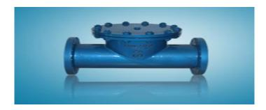
Tee strainer is fabricated from pipes & plates or standard equal tee & flanges. Filter elements are made of stainless steel perforated sheet or wire mesh supported by perforated sheet. In tee type strainer many times a structural skeleton made of flats and round bar is used to support the wire mesh. Tee Type Strainers are a low cost solution to large nominal bore straining requirements Tee strainers feature either bolted cover or quick opening covers for application suitability.
